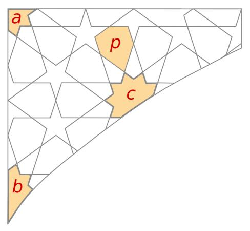
Fig. 12: The scheme of the upper-level pattern on the left spandrel of the Masjid-i Seyyed. The locations of the central stars a, b and c are marked. Area p is the petal which had to be inadvertently expanded slightly, because of a misplaced level-1 band to its right.
